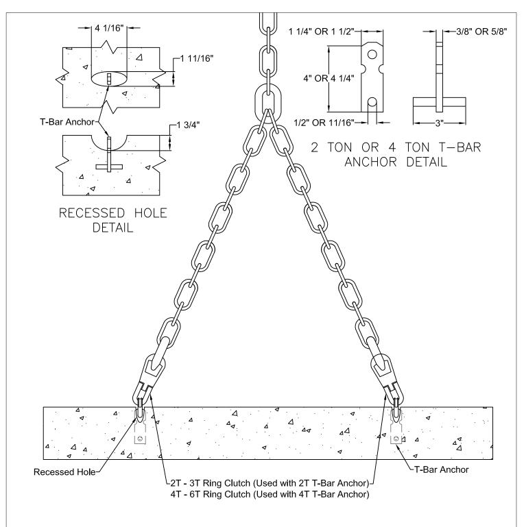
\*Recommended Lifting Equipment: Heavy—duty three—way chains with self—locking hooks.
