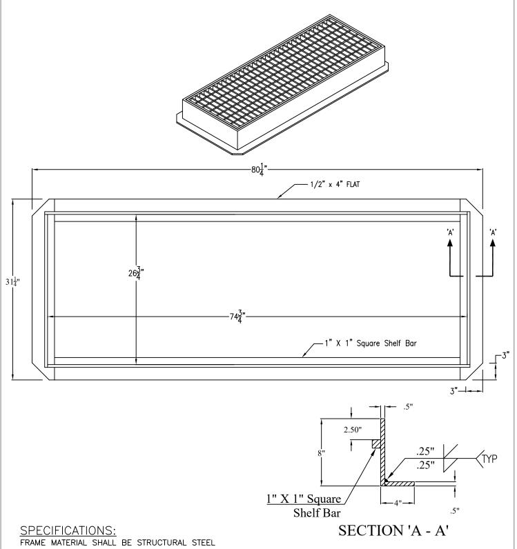
FRAME MATERIAL SHALL BE STRUCTURAL STEEL CONFORMING TO ASTM A709 GRADE 36 STEEL. FRAME TO BE PAINTED WITH ONE COAT OF BLACK BITUMINOUS PAINT IN ACCORDANCE WITH PENNDOT PUBLICATION 408.
