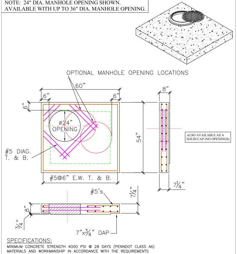
OF PENNDOT PUBLICATION 408 SECTION 605 & 714 STEEL REINFORCEMENT A615 GRADE 60 HORIZONTAL AND VERTICAL
