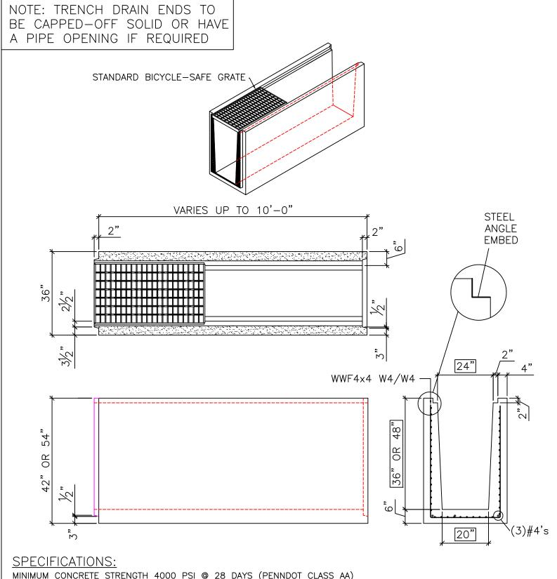
MINIMUM CONCRETE STRENGTH 4000 PSI @ 28 DAYS (PENNDOT CLASS AA) MATERIALS AND WORKMANSHIP IN ACCORDANCE WITH THE REQUIREMENTS OF PENNDOT PUBLICATION 408 SECTION 605 & 714 STEEL REINFORCEMENT A615 GRADE 60 HORIZONTAL AND VERTICAL
